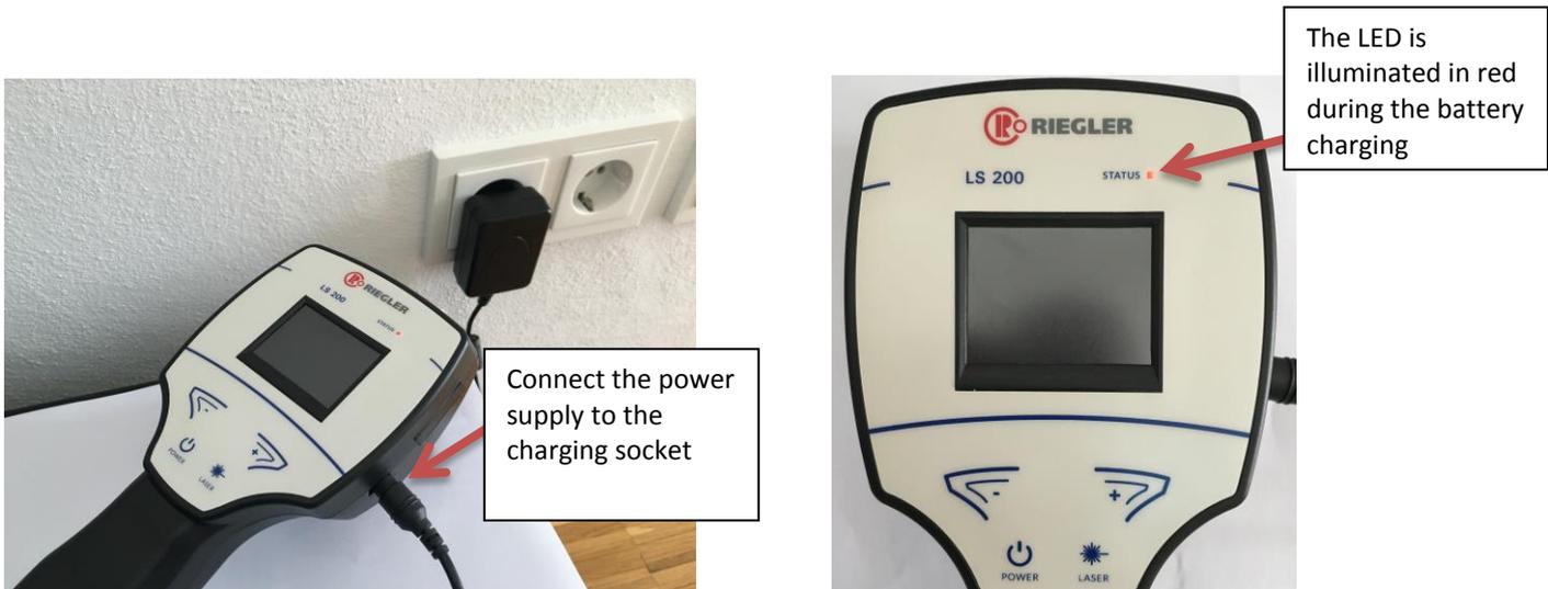
The LS 200 checks the charge status of the battery and automatically starts the charging process. The following scenarios are possible:
